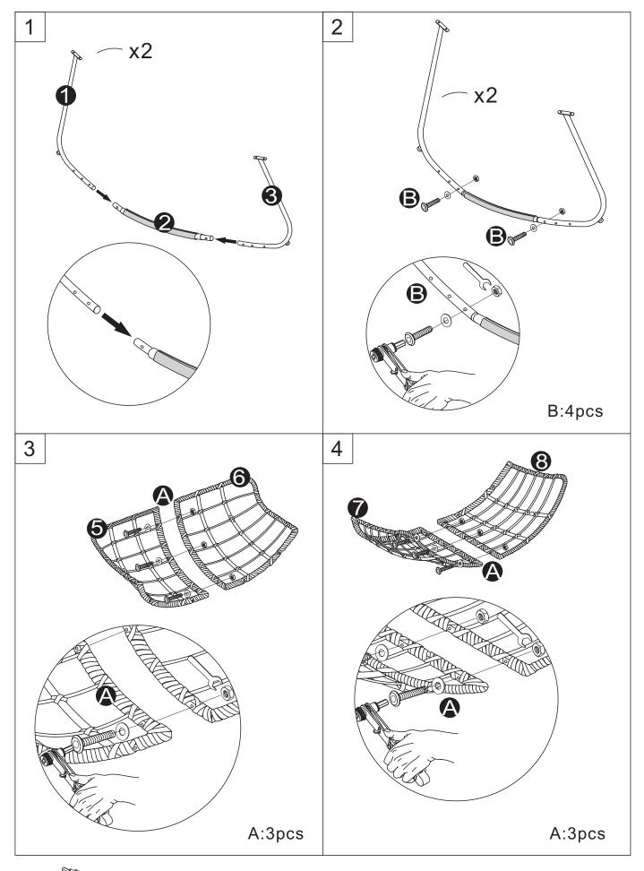
Notice: Install relevant screws, don't tighten completely at beginning Alignment & Tighten fully when you complete the seat base section.
